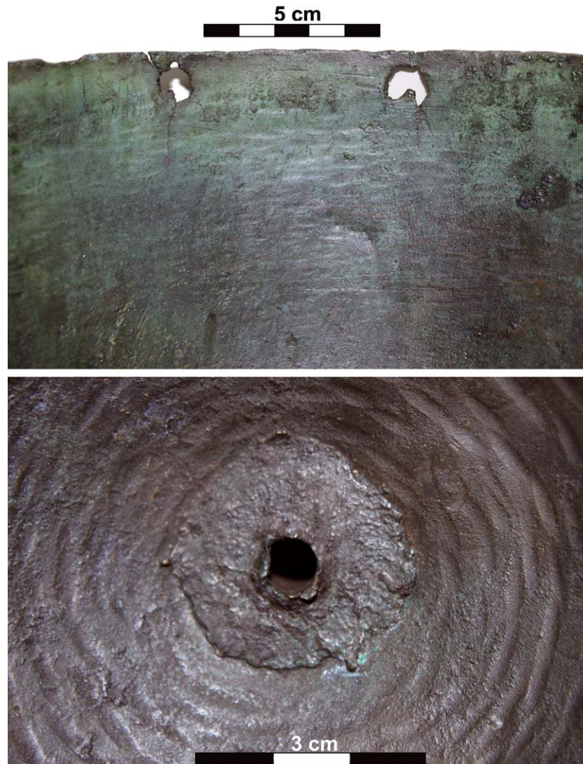
Fig. 2.3 Hammering traces on the inside of the helmets of Type Pișcolt from Șoarș, Romania (above) and Pișcolt, Romania (below).
